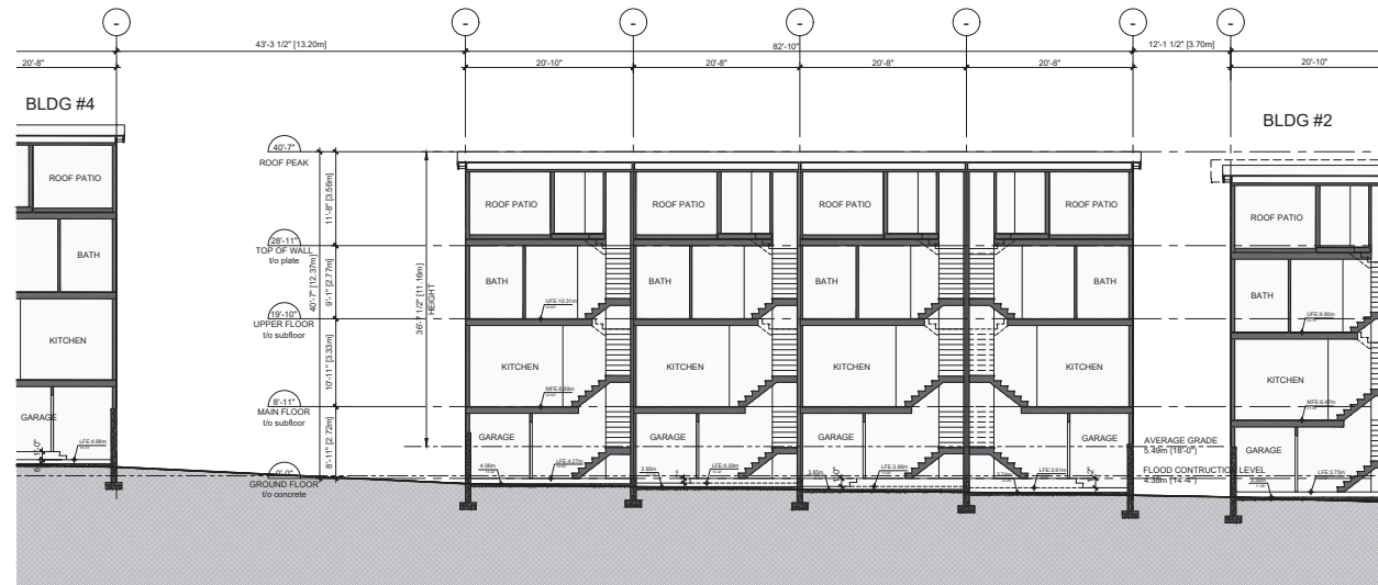
3 SECTION - BLDG. #3 A3.32 SCALE 1/8" = 1'-0"
