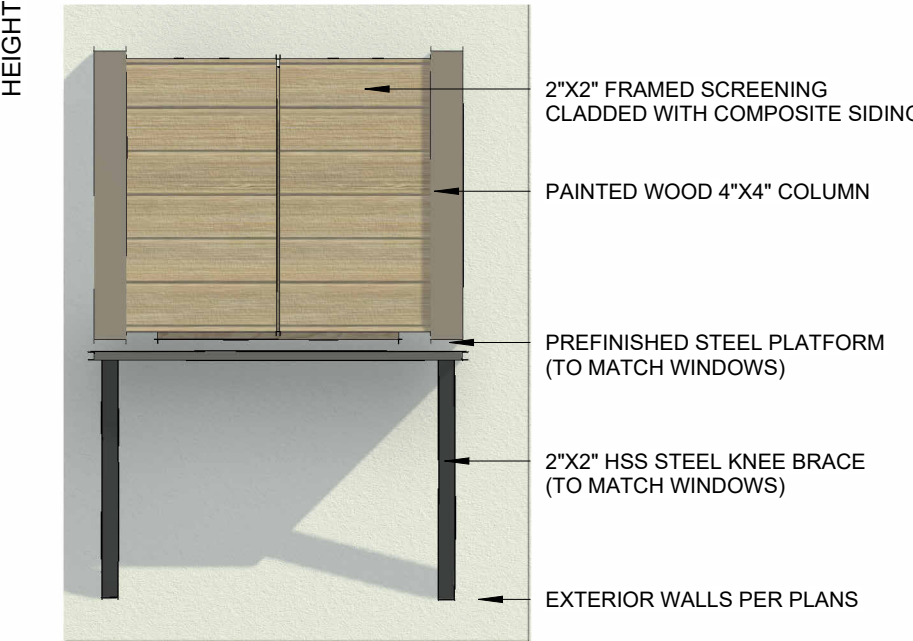
4 Heat Pump - Screening (Front) 1/2" = 1'-0"
