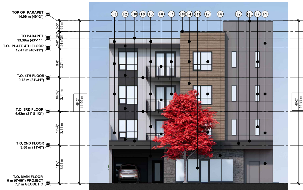
1 EAST ELEVATION AT THIRD STREET SCALE: 3/16" = 1'-0"
