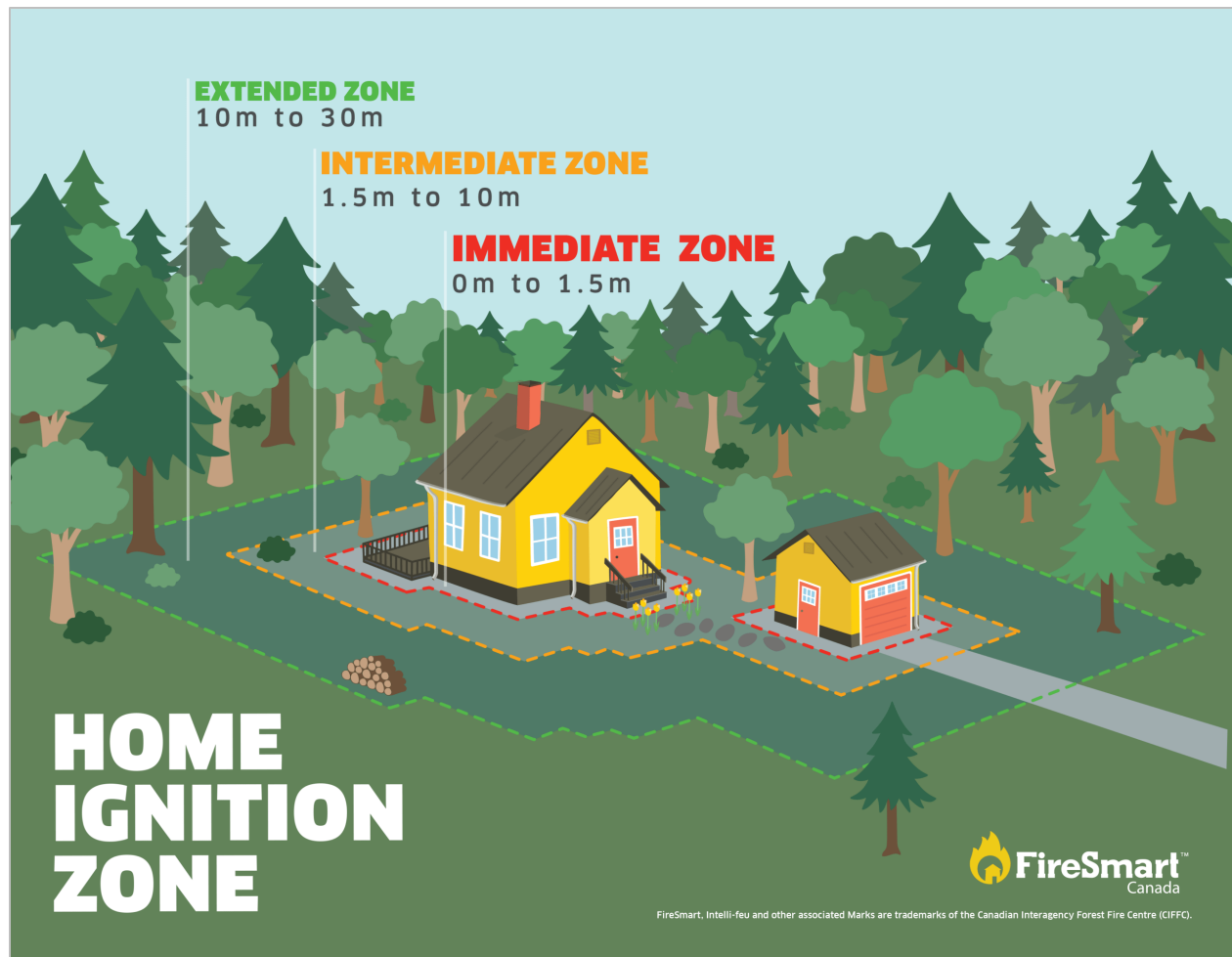
Figure 13. The FireSmart zone system.
