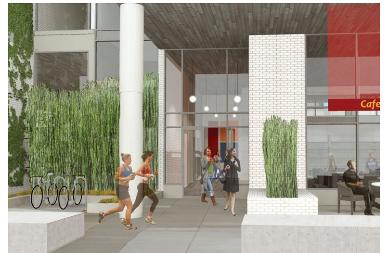
Figure 5b: An example of a residential entrance facing the principal frontage street, differentiated and separated from adjacent retail, restaurant, or commercial uses
