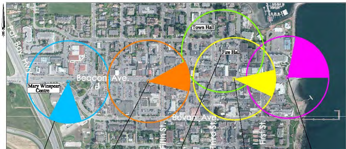
MARY WINSPEAR Lamp Standard - HIGH-LOW Access Point - MOTOROLA AP7181 Camera - AVIGILON HD H.264
