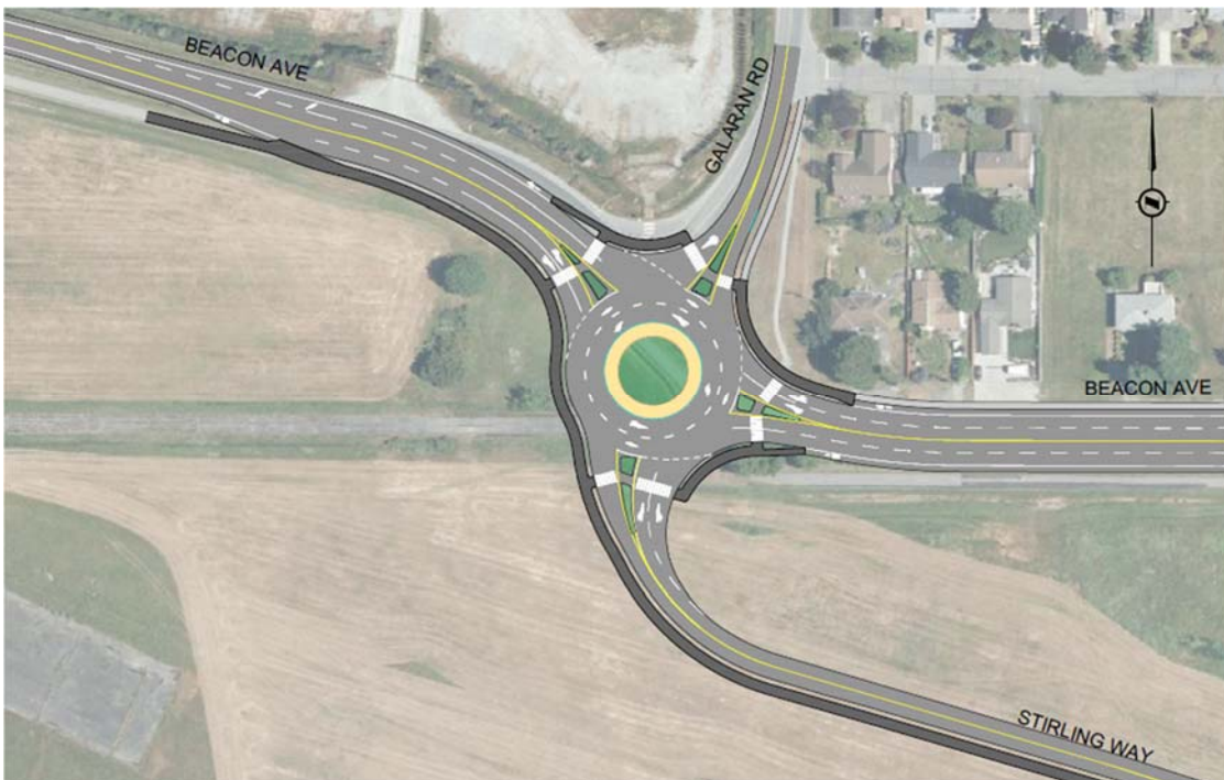
Concept sketch of a two-lane Beacon Ave / Galaran Rd / Stirling Way roundabout and Stirling Way realignment.
