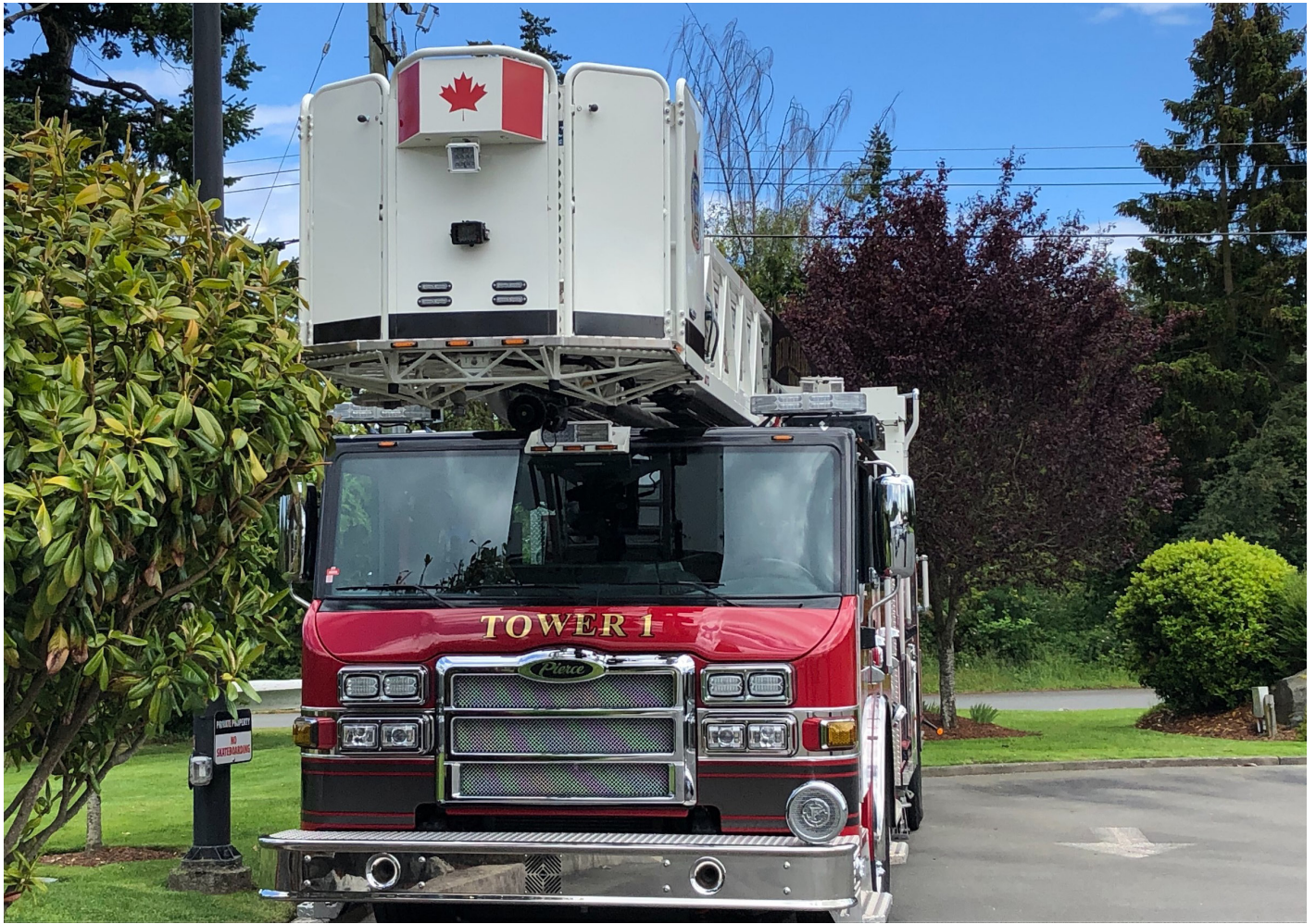
||| Sidney's new tower ladder truck has a bucket at the end of the ladder that can move from window to window collecting people during an emergency evacuation.
