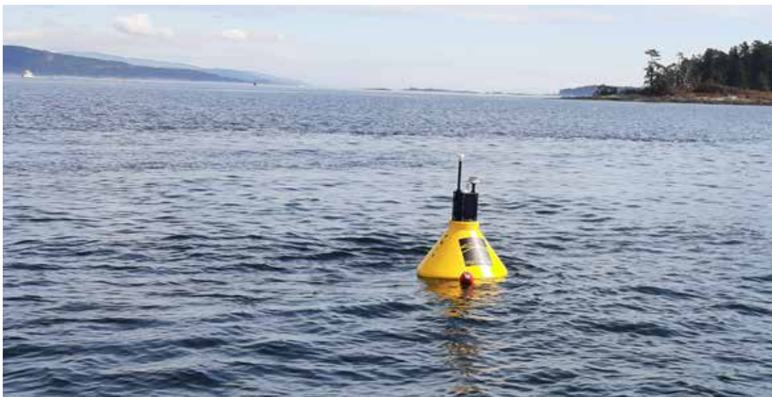
Two data collection buoys in Haro Strait have been informing refined flood risk modelling.
